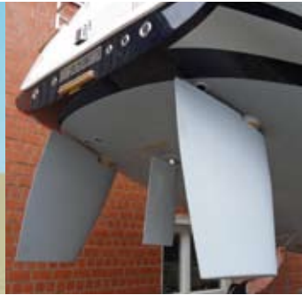
The lead ballast swing keel delivers perfect performance and stability and three rudders ensure easy manoeuvrability
