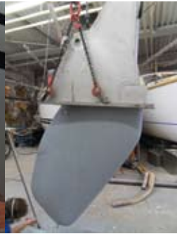
The lead ballast swing keel delivers perfect performance and stability and three rudders ensure easy manoeuvrability
