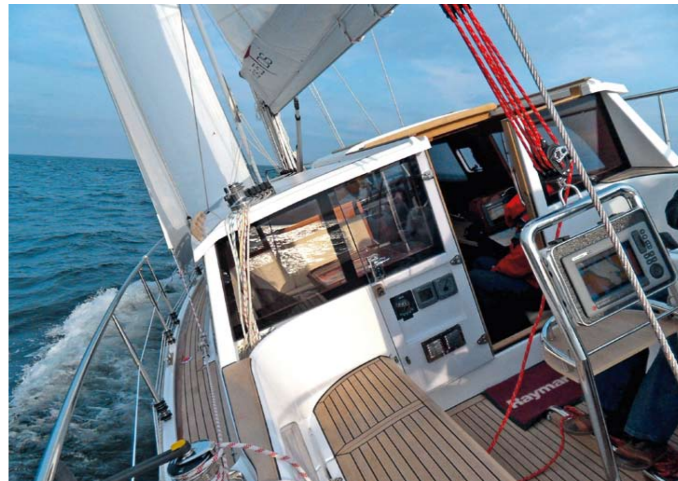
The Sirius 35DS in her element. Note the neat, midships mainsheet horse, sturdy steel guardrails and useful halyard stowage
